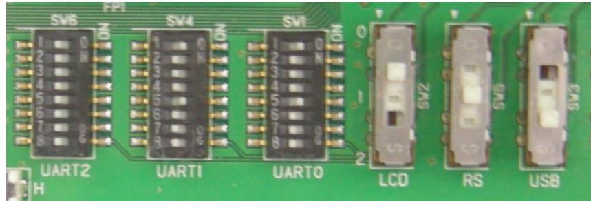
The terminals for using UART can be selected by DIP switch (SW1, SW4, and SW6).
